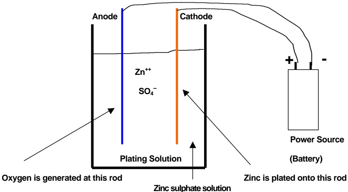
This simple plating cell illustrates the actions during the plating process. At the cathode (steel, for example), zinc ions dissolved in the zinc sulphate solution combine with 2 electrons and form elemental zinc. The zinc deposits onto the cathode surface. At the anode, water is converted to oxygen and hydrogen ions to maintain electrical balance. The oxygen forms as a gas; thus, nothing is deposited on the anode surface. The plating solution carries the current between the cathode and anode.
